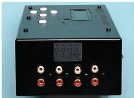
End-on and side-on views showing the eight inputs (left); above is the DC in/out, games port socket, serial socket, invalid MIDI LED and MIDI output
