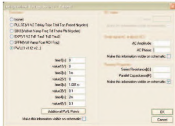
Fig.3. Selecting the PWL function for a voltage source
