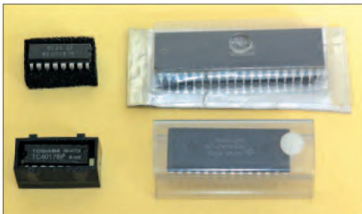
Fig. 1. Four types of anti-static packing. Clockwise from top left-hand corner they are: conductive foam, blister pack (with conductive backing), plastic tube, and conductive plastic holder
