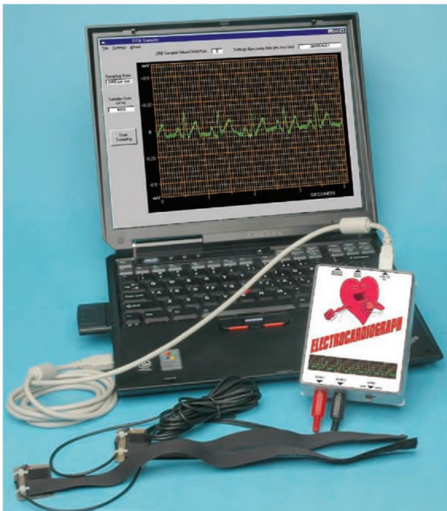
The complete ECG setup using our Electrocardiograph, a laptop PC (with USB) and home-made electrodes. You can also use commercial ECG pads.
