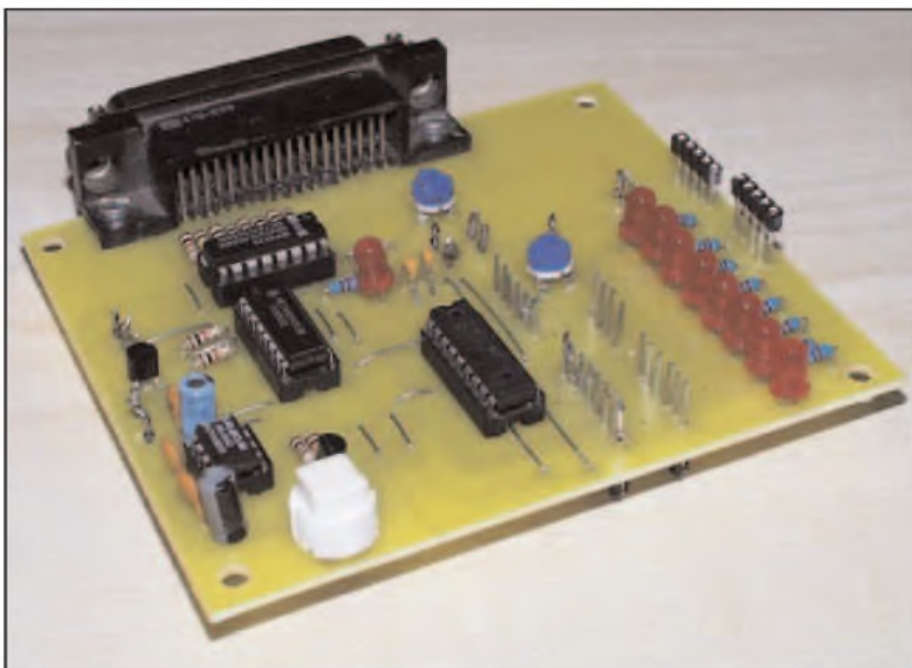
Prototype of the dual-purpose PIC programming and development interface board used in the Teach-In 2008 series
