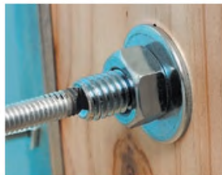
The lower pivot point is formed by first grinding the end of the bar to a sharp edge. This sharp edge then rests vertically against the end of a 13mm x 40mm-long bolt.
