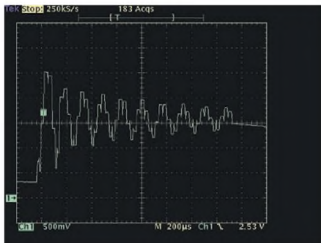
Fig.7c: with a timebase of 200 \mu s/div, the sample-and-hold control signal is now just a succession of spikes and is not shown. At this time scale, the sequence of flat plateaus reproduces a digitised version of the original ringing waveform of Fig.7a, occurring at a rate almost 1000 times faster.
