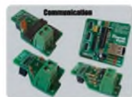
CAN-1 Board - Interface CAN via MCP2551
