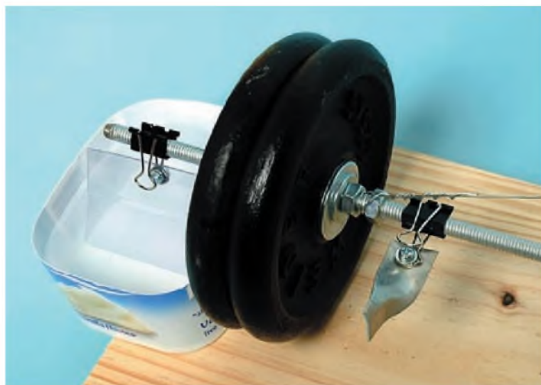
Above and right: these two views show the alternative damping methods for the swinging bar. Magnetic damping (above) uses a couple of super magnets and a coil of wire, while liquid damping (right) uses a 40 x 50mm plastic paddle dipped into a rectangular container of water.
