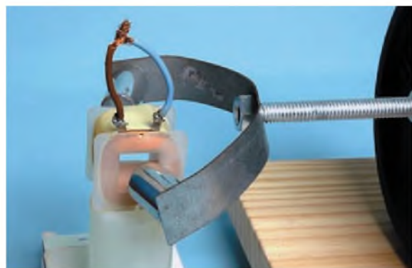
Above and right: these two views show the alternative damping methods for the swinging bar. Magnetic damping (above) uses a couple of super magnets and a coil of wire, while liquid damping (right) uses a 40 x 50mm plastic paddle dipped into a rectangular container of water.
