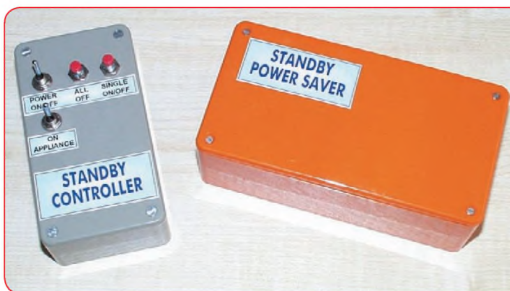
The completed prototype transmitter (left) and receiver (right) modules that make up the Standby Power System. Not shown on the receiver unit are the Main ID and Unit On/Off pushbutton switches (S6 and S7)
