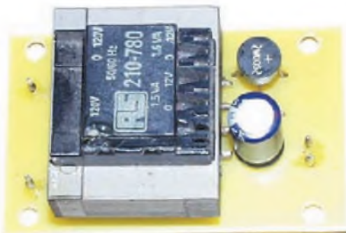
Fig.6. Circuit board details for the optional mains power supply
