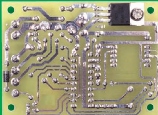
This view of the copper side of the PC board shows how REG1 and D3 are installed.
