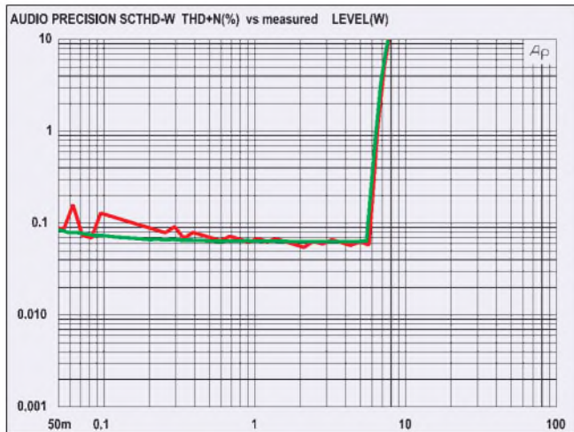
Fig.4: THD + noise vs. output power into 4Ω. The right channel (red) has higher distortion at the lower power levels due to noise from the power supply circuitry.
