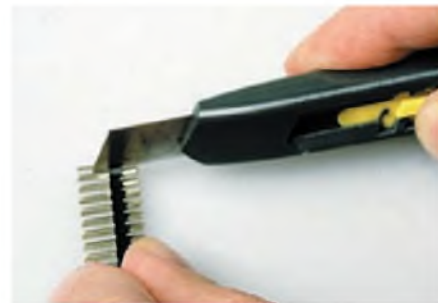
You can easily make 2-way and 4-way pin headers for JP1 and JP2-3 by cutting down a longer strip.
