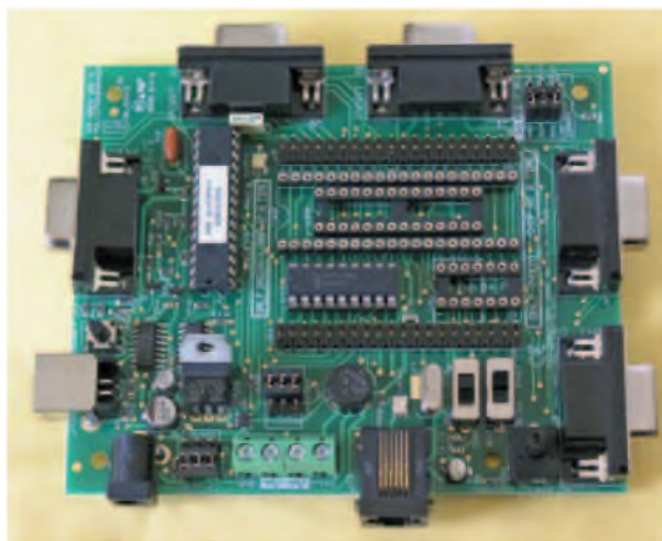
Fig. 1: The Multi-programmer has sockets to accommodate a wide range of PIC chips. It can also be used as the basis of a PIC prototyping system
