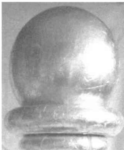
Discharge terminal "ball".
