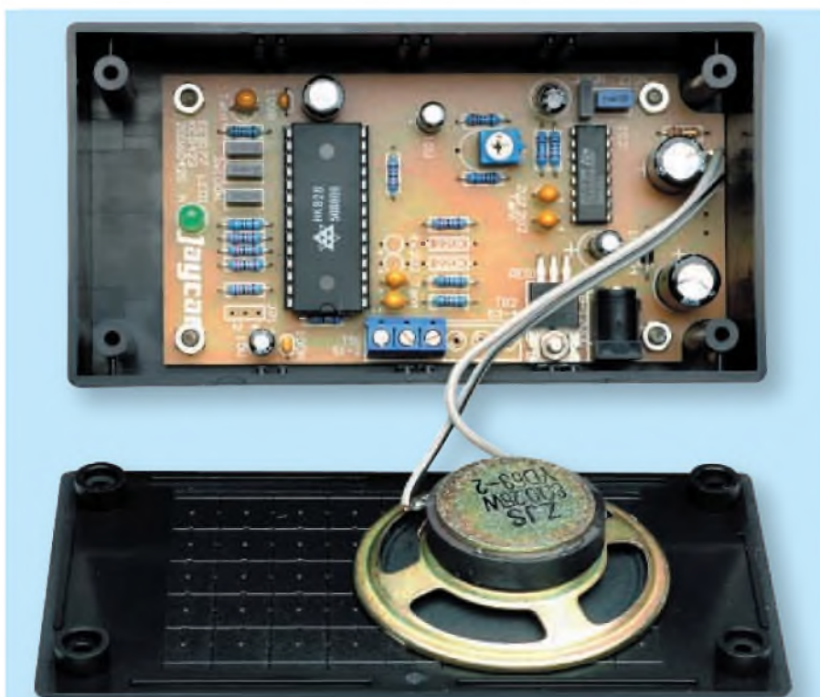
Fig.2: the circuit board fits neatly inside a standard UB3-size plastic case, and is secured using M3 × 10mm machine screws and nuts – see text. The loudspeaker is secured to the lid using epoxy adhesive.
