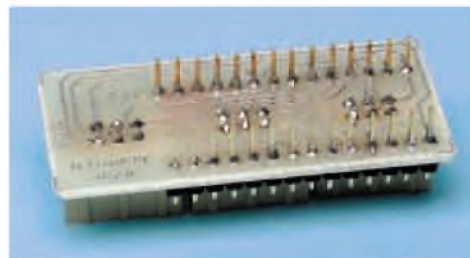
This view shows how the 28-way header pins protrude through the PC board.
