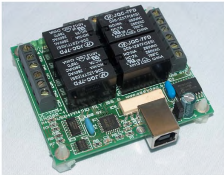
Fig.4. Although it connects to a USB port, this EasyDAQ board can be controlled as if it was connected to a standard serial port. This probably represents the simplest method of USB interfacing
