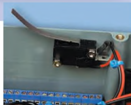
The microswitch is mounted about 7mm below the lip of the case. Bend its actuating arm upwards as shown, so that the switch is held open when the lid is in place.
