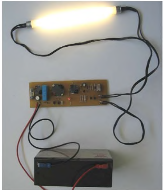
Testing the operation of the PCB prior to casing up
