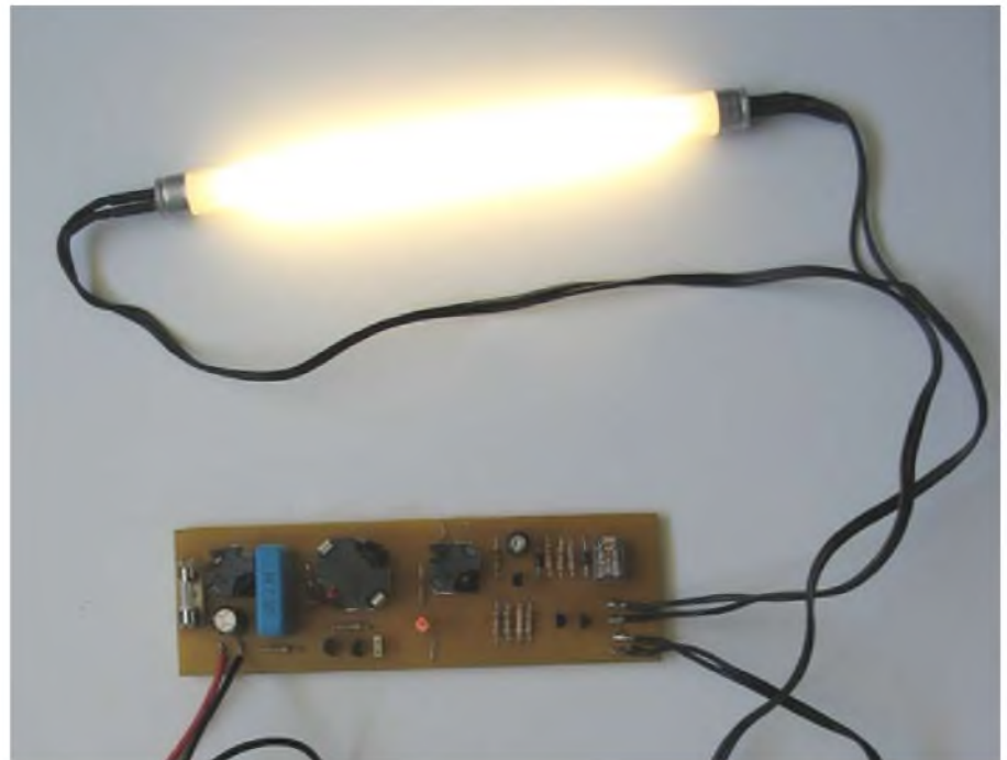
Fig.2: Basic sinewave resonant converter circuit
