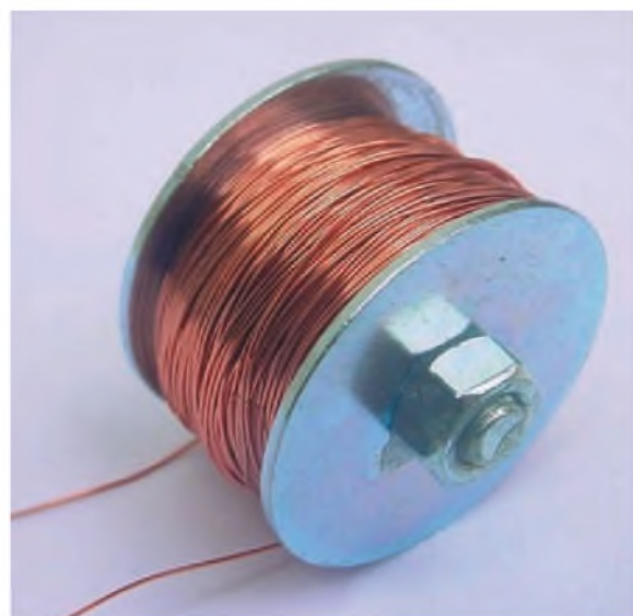
Construction of the sensor coil L1. Approximately 1,200 turns of 30swg/22awg enamelled copper wire are wound on a 6mm x 25mm long bolt
