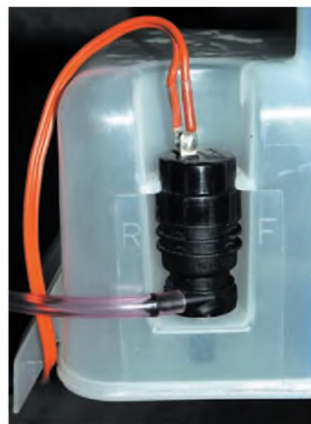
A simple pump/reservoir combination for an intercooler water spray can be cheaply obtained by using a windscreen washer reservoir and pump.
