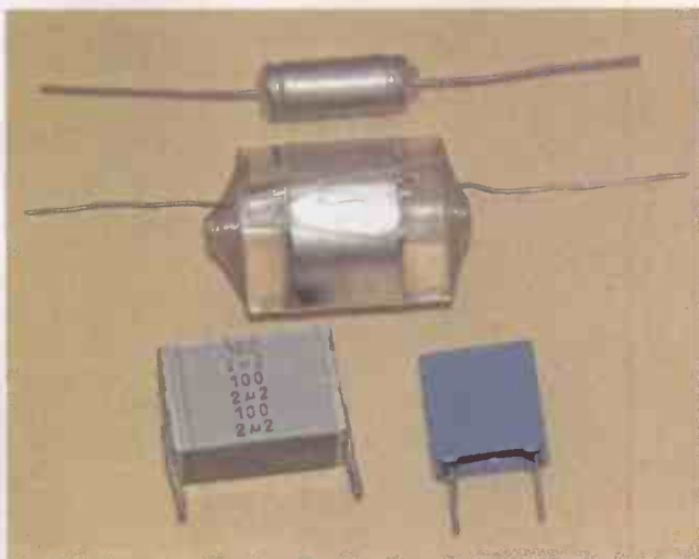
Fig.1. Axial lead capacitors (top and middle) are used relatively little in modern projects. PC capacitors (bottom) are now the norm
