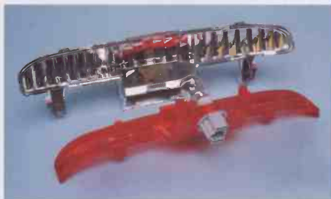
(2). Once we had the assembly on the bench, it was a simple matter to separate the red lens from the reflector to get to the insides. Be careful with the clips that hold these parts together, as the plastic is very brittle.
