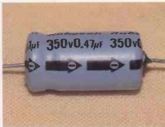
Fig.2. An indentation around the body indicates the positive end of an axial electrolytic capacitor. The "-" and (or) "+" legends are normally included as well
