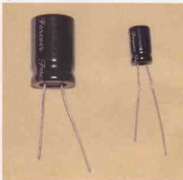
Fig.3. PC electrolytic capacitors usually have one lead shorter than the other. The shorter lead is the negative (-) one
