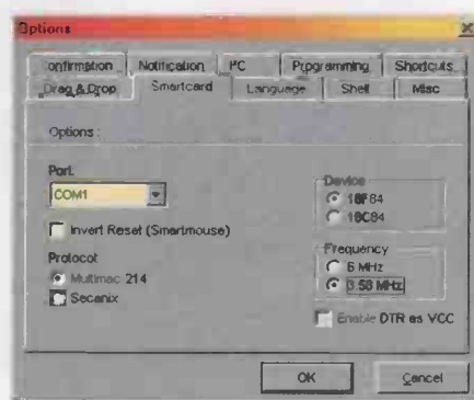
Fig.6: the default values for IC-Prog's smart card settings. Not all cards support the 6MHz clock rate, so select the "3.58MHz" setting for maximum reliability. Jumper JP2 on the PC board should be set to agree with the frequency selected here.
