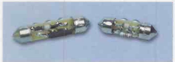
The completed festoon lamp assemblies can be plugged straight into a conventional festoon lamp holder but must be oriented with the LEDs facing outwards.
