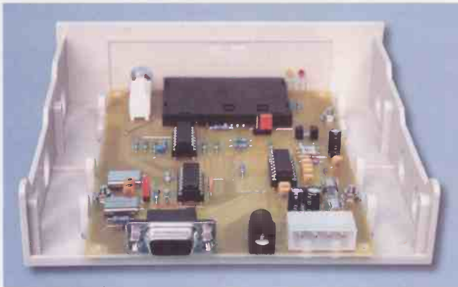
This view shows how the PC board is fitted to a standard 3.5-inch to 5.25-inch drive mounting kit. We cut down an old 5.25-inch drive blanking plate to fill the hole in the front of the adapter.
