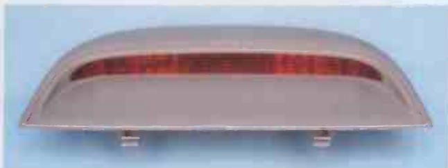
(1). The Accord's CHMSL sits on the parcel shelf and is retained with two clips accessible from within the boot space. The entire assembly came away in less than 10 seconds!
