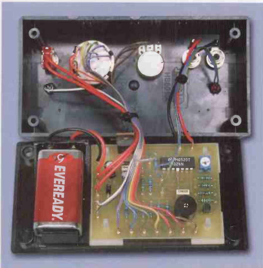
The PC board and battery holder are mounted on the lid of the case, as shown in this photo (see text). Use several cable ties to keep the wiring neat and tidy but leave enough slack in the wiring so that the lid can be opened out.
