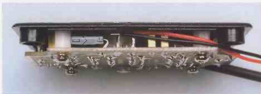
The close-up view shows the completed assembly, just before it is fitted to the case. The flash trigger lead emerges through a small semicircular notch near the top centre of one side of the jiffy box.
