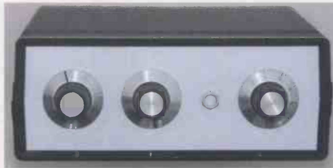
Fig.1. Producing a dummy front panel layout gives a good idea of what the finished project will look like
