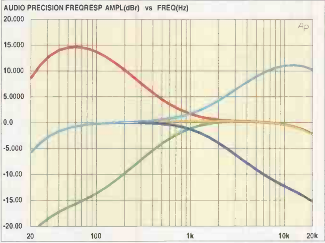
Fig.8: the tone control action in the “flat”, “max boost” and “max cut” settings.
