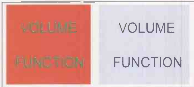
Fig.3. Good colour contrast (left) does not necessarily produce text that is easy to read. High tonal contrast (right) usually provides good legibility
