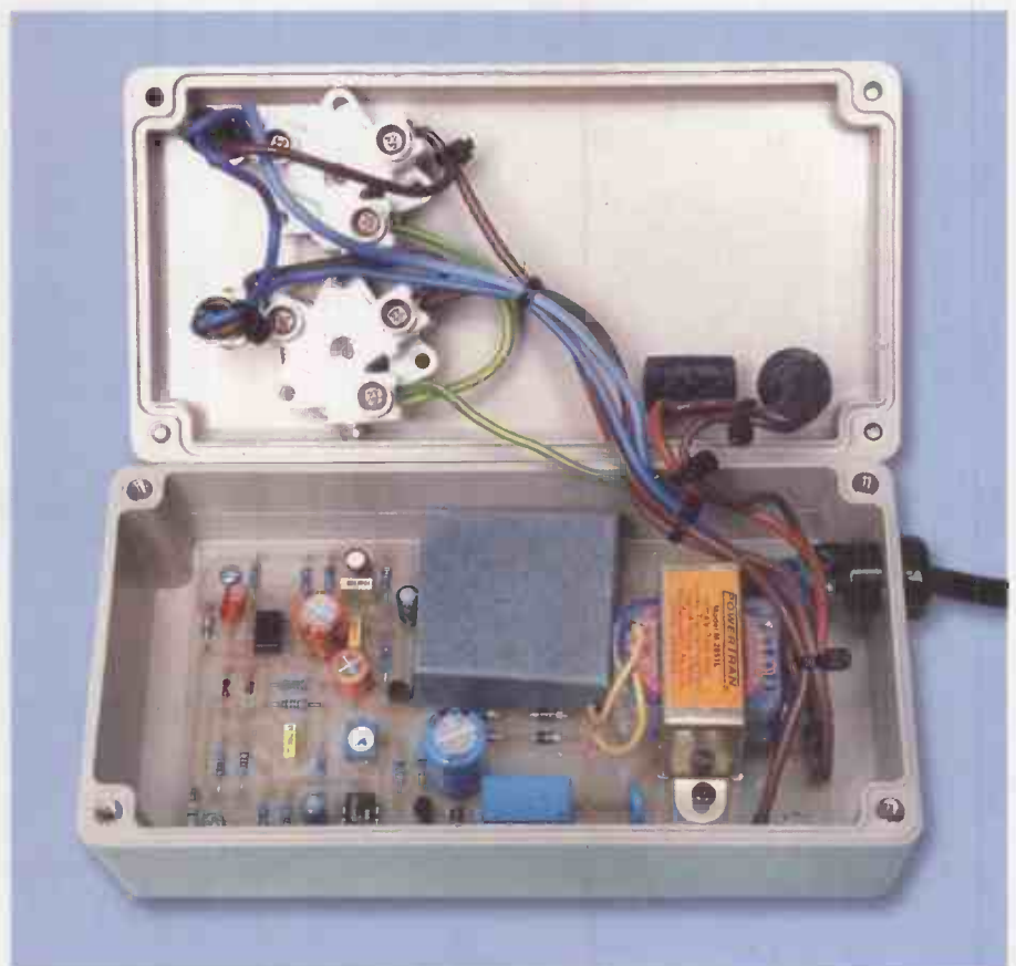
This is the view inside the prototype. The toroidal coil on the PC board operates at mains potential and is protected by a plastic insulation cover (see text).
