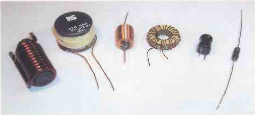
Photo 5.1. Various inductors with values ranging from 10μH to 1mH at current ratings from 100mA to 25A
