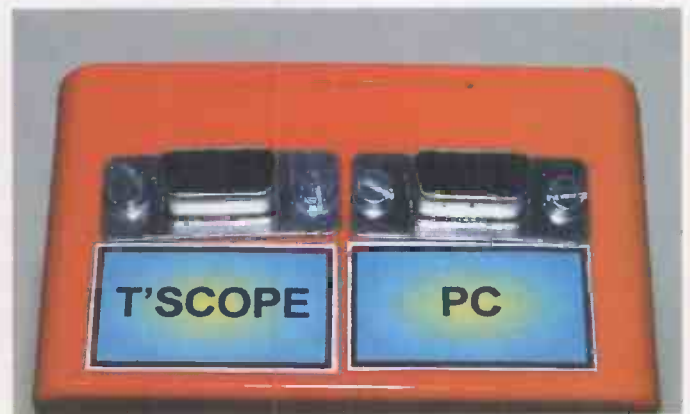
The two ends of the case showing the GPS input socket and the Telescope and PC serial connectors
