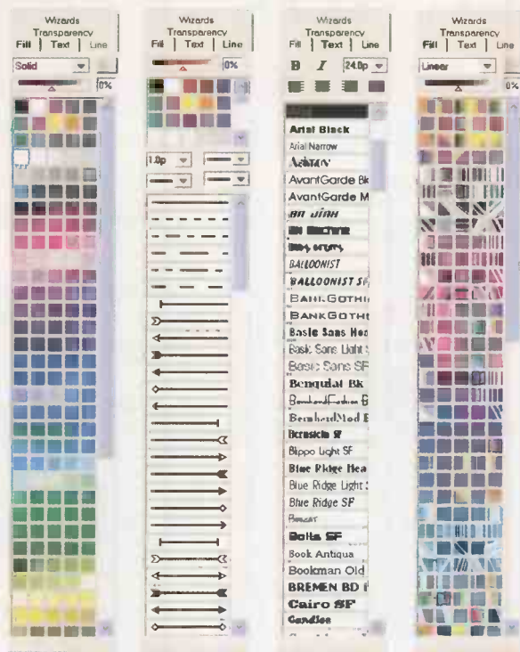
Fig.2. Serif DrawPlus 4 has a tabbed control panel that provides numerous line and fill options, plus a range of text features. Graduated fills (extreme right) are available but are best used sparingly
