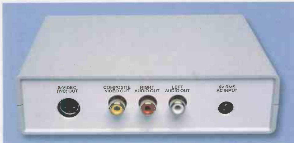
The A/V output sockets are all accessible from the rear of the unit. They include a 4-pin mini-DIN socket for the S-video signals, plus three RCA sockets for the composite video and left & right channel audio output sockets. The socket at far right is the DC power connector.
