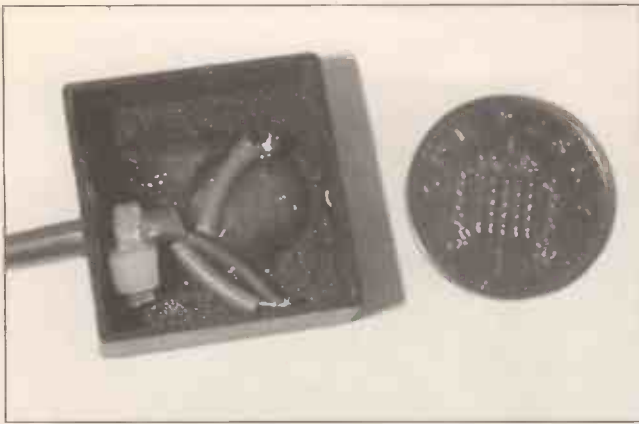
The light-dependent resistor (l.d.r.) is pushed into a hole in the light sensor box and secured in position using quick-setting epoxy adhesive.
