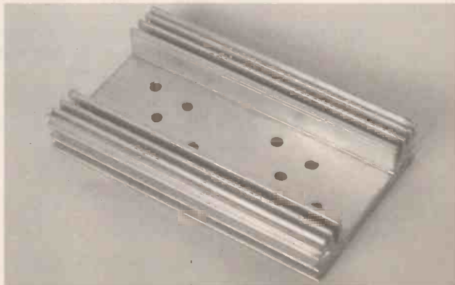
Fig.3. An extruded aluminium heatsink drilled to take two TO3-cased devices.
