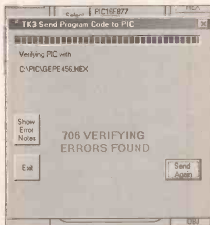
Photo 13. Programming sub-screen following detection of programming errors (image simulated for sake of illustration - you are unlikely to experience verification errors).
