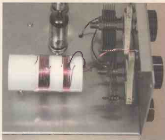
Fig.3. Details of the home-made tuning coil. The plastic coil former measures 32mm diameter by about 65mm length. Strips of tape can be used to stop the windings unravelling – see photograph right.
