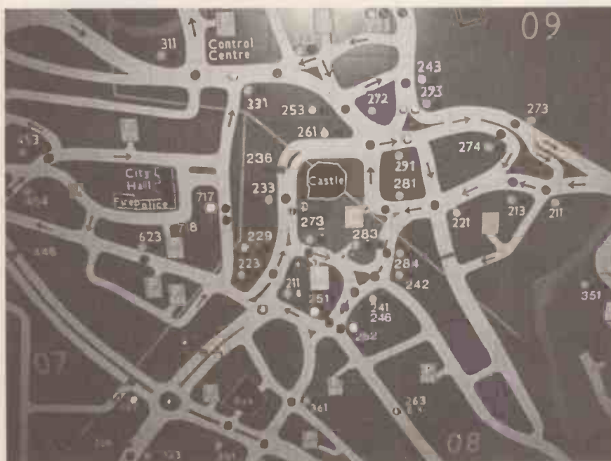
Fig.3. The control room of the Norfolk UTCC has a large-scale map showing the current state of all the traffic lights in Norwich, including pedestrian crossings.
