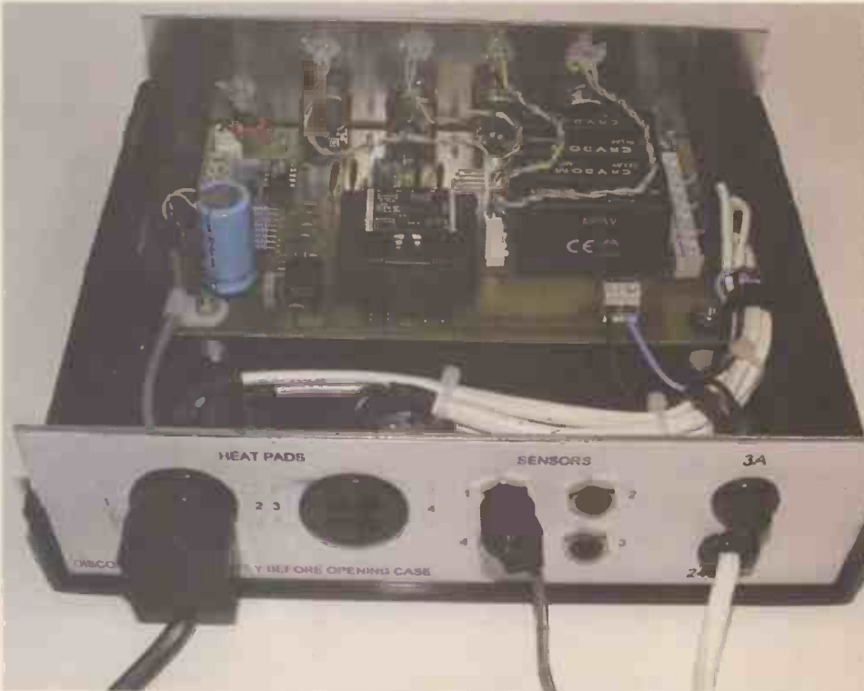
The rear panel sockets, fuse and mains cable positioning.
