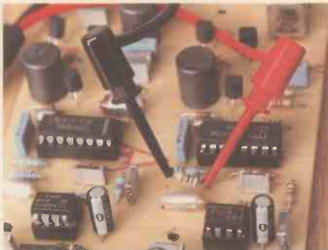
Fig.3. Semi in-circuit testing of a resistor.
