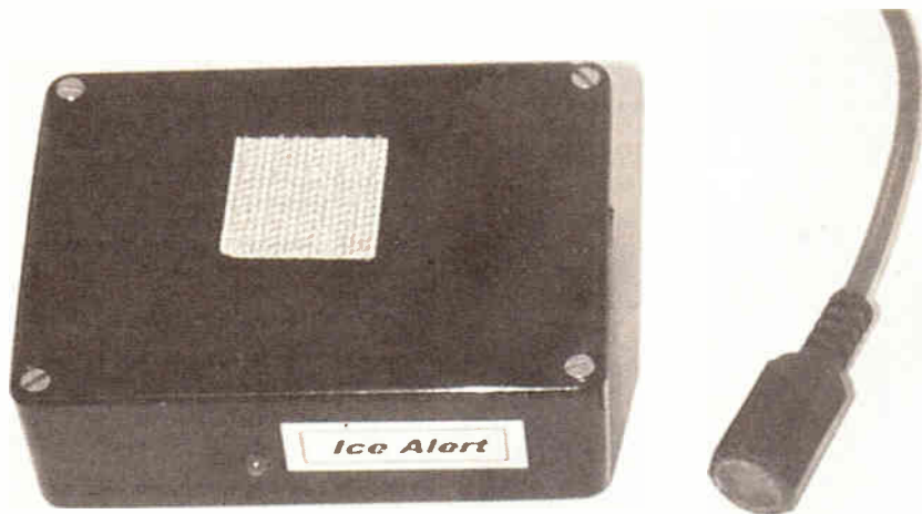
Completed Ice Alert. The small square of Velcro enables it to be easily installed below a vehicle dashboard.
