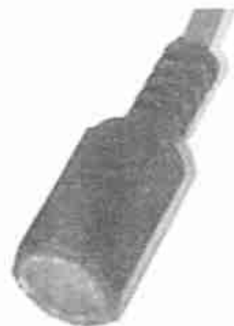
The bead thermistor temperature sensor encased in a phono plug.
