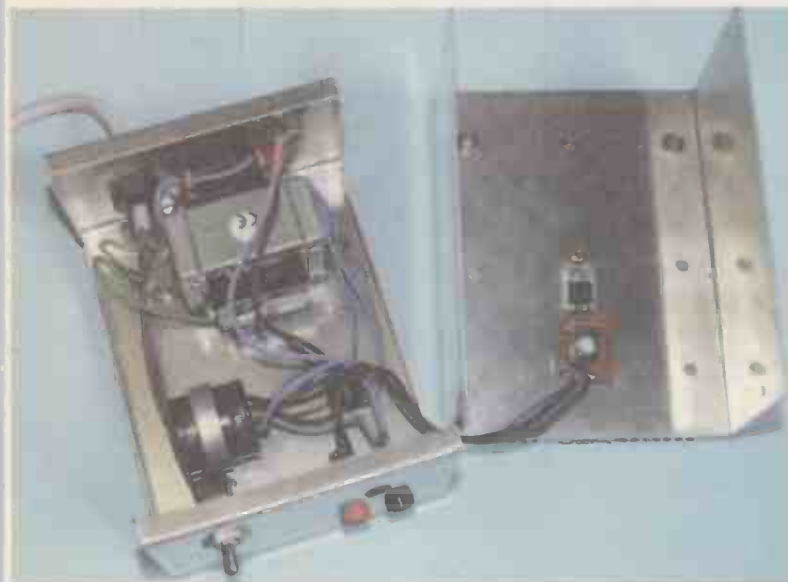
General component layout within the aluminium case. Note the regulator and small circuit board mounted on the underside of the case cover.
