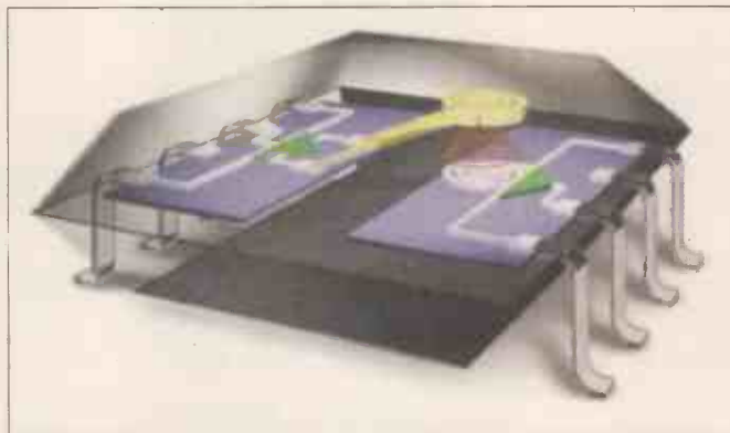
MEMS devices offer circuit isolation using high speed magnetic techniques. (Illustration courtesy Analogue Devices)
