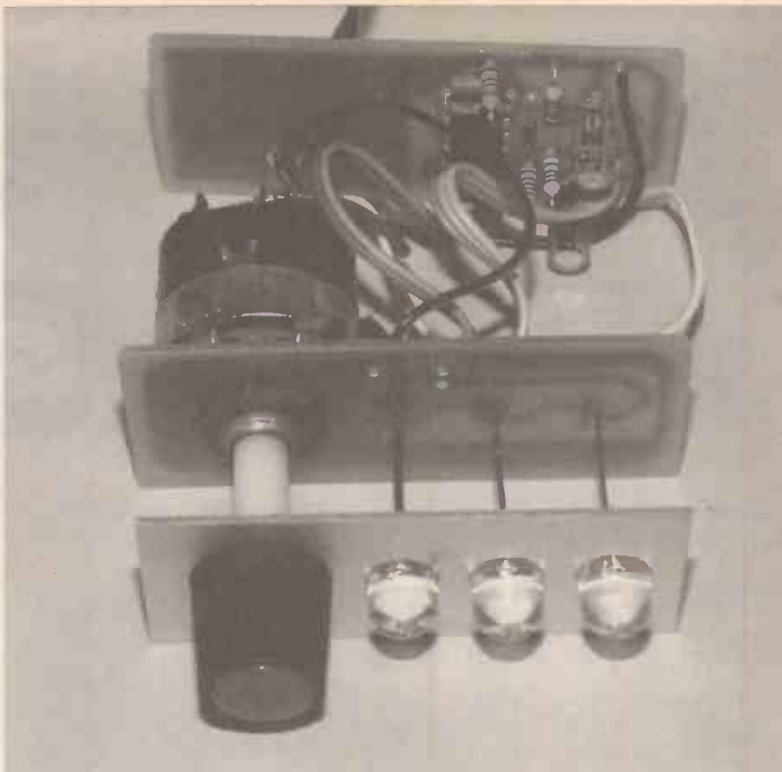
The "sandwich" of p.c.b.s and front panel removed from the case showing the method of mounting the l.e.d.s by using the full length of their leads.
