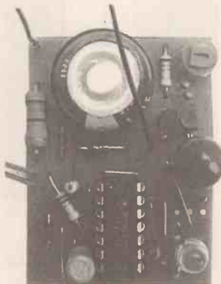
Completed "touch-light" circuit board.
