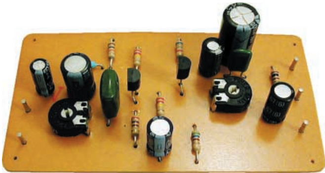
Completed p.c.b. for the Low-Noise Preamplifier.
