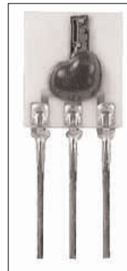
Fig.1 (above). Internal elements and construction of the HIH3605 capacitive RH sensor.
