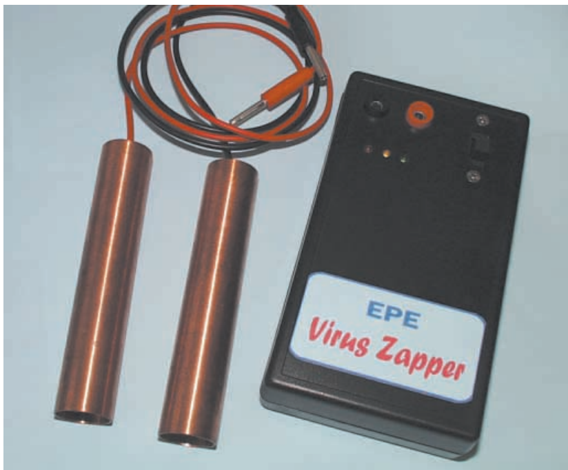
Completed PIC-based Virus Zapper together with copper tube electrodes.
