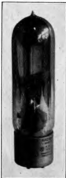
Fig. 74. — Illustrating Radiotron; UV-203; a 50-watt power tube.
