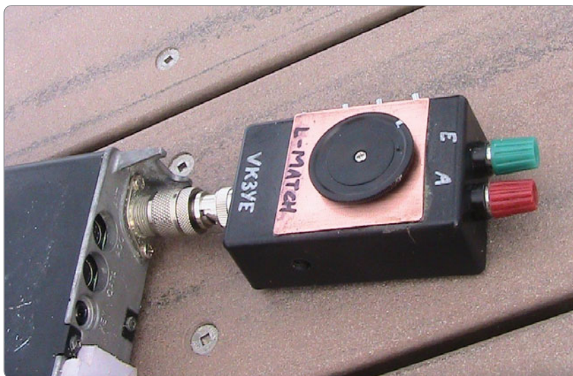
Photo 4: Antenna coupler – in use.
