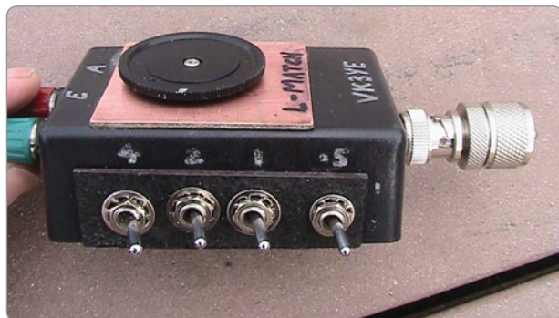
Photo 1: Antenna coupler – top.
