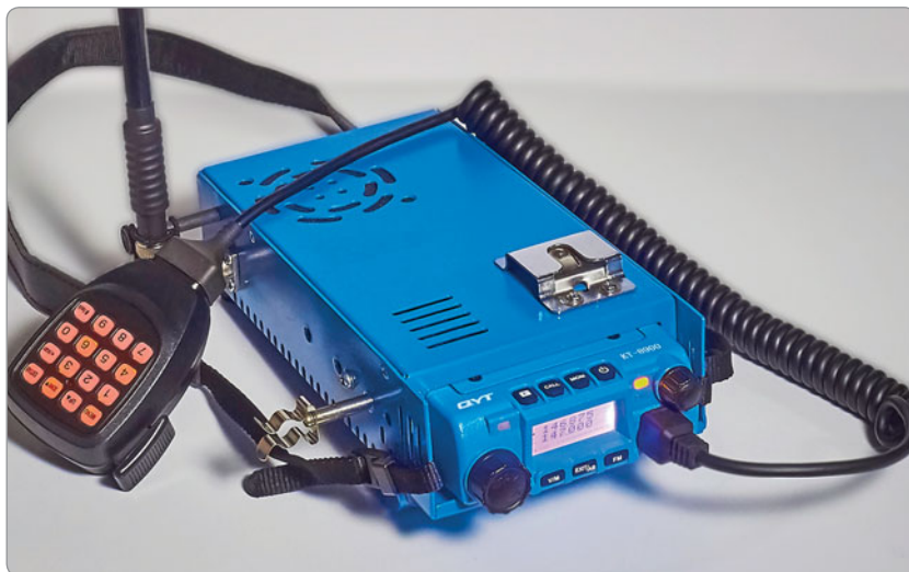
Photo 4: Radio operates well with telescopic dual band antenna. To avoid scratches, add heat shrink tubing to the area where the antenna clips back in to side of case.
