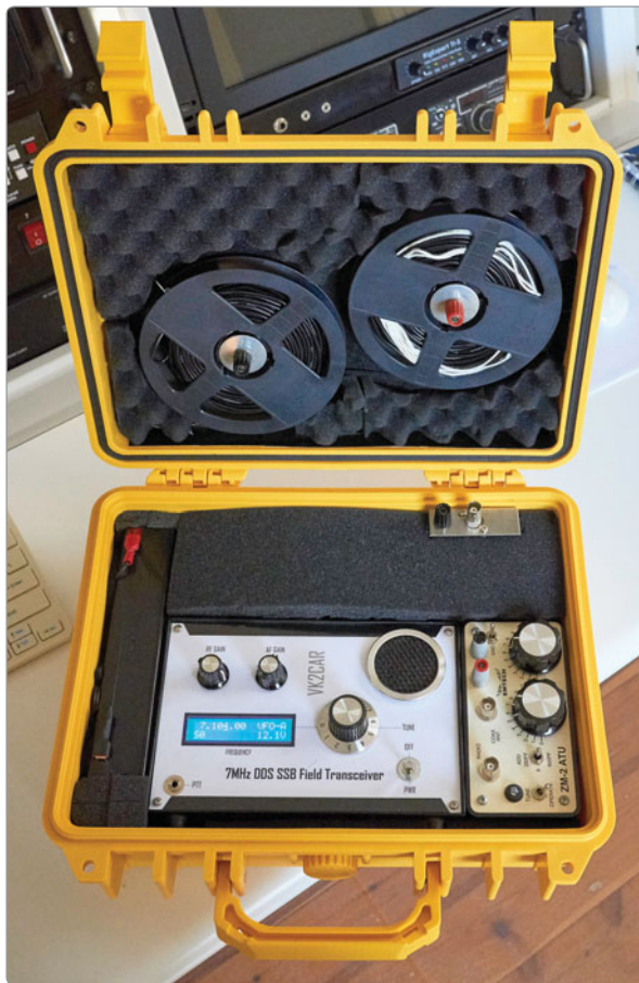
Photo 5: Complete 40 m SSB transceiver with antenna and z-matcher (mic and leads tucked under foam) ready to go SOTA.
