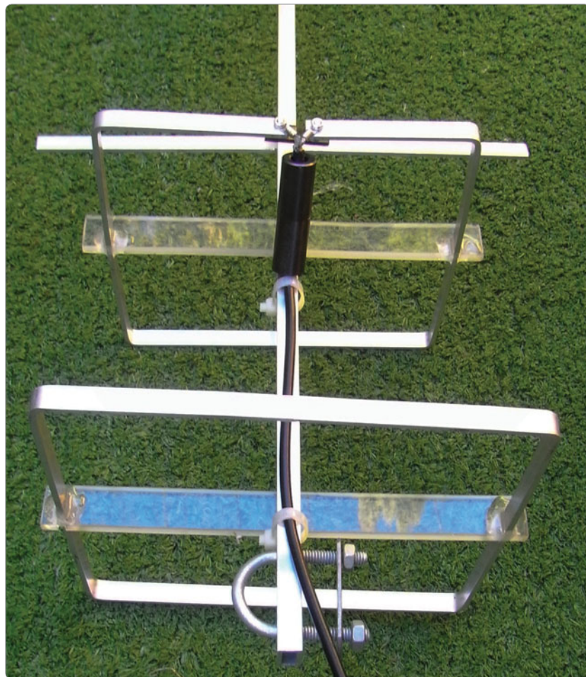
Photo 4: The coaxial cable routed through two ferrite sleeves to the feedpoint.
