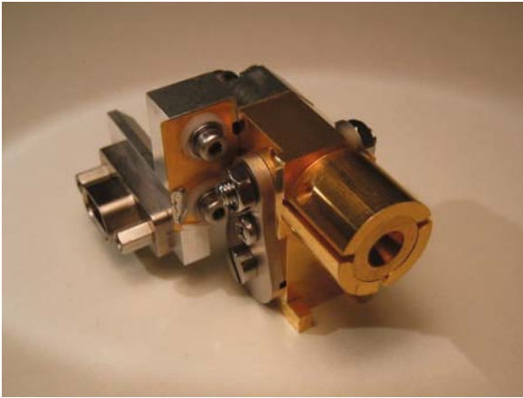
Fig. 5.12 [An ALMA Band 9 SIS mixer] A photo of the feed horn on the right, and the SIS mixer holder on the left. This was built at the Space Research Organization of the Netherlands (SRON). This receiver covers the frequency range 610–720 GHz. This is a tunerless double sideband mixer. This is typical for the sub-mm SIS mixers used in the ALMA instrument
