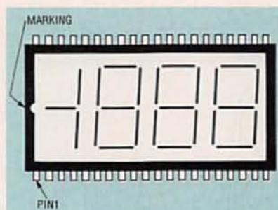
FIG. 7—THE LCD MODULE has a marking similar to that on an IC, indicating where pin 1 is. Note that the module mounts on the solder side of the digital board, so be careful where pin 1 goes.
