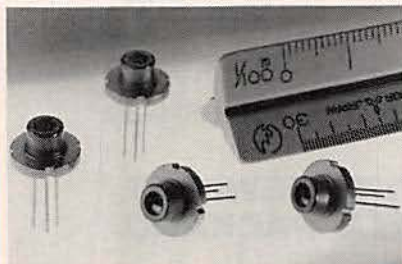
OSCILLATING AT WAVELENGTHS between 800 and 870 nm, Sanyo's high-power lasers will have applications in optical-disc memories, satellite communications, and blue-laser light generation.
