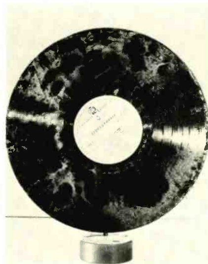
FIG. 5—UNTREATED RECORD after being exposed in dust chamber.
