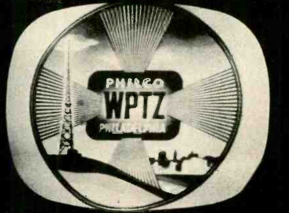
Appearance of screen when cosine yoke is used without the corrector magnets.
