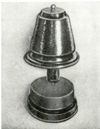
Photo of the capacitance-operated lamp. It is all metal and the circuit components are mounted in the large base.
