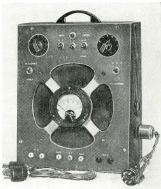
At left is a front panel photo of the portable loudspeaker test unit. Above is a rear view of the unit.
