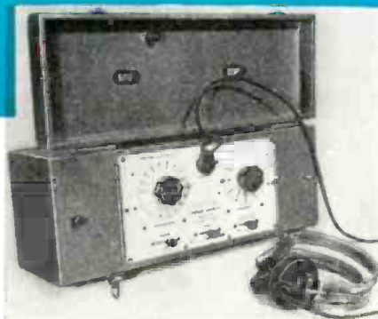
Photo of a screening audiometer. Compact units like this are used by nurses to check the hearing of schoolchildren.
