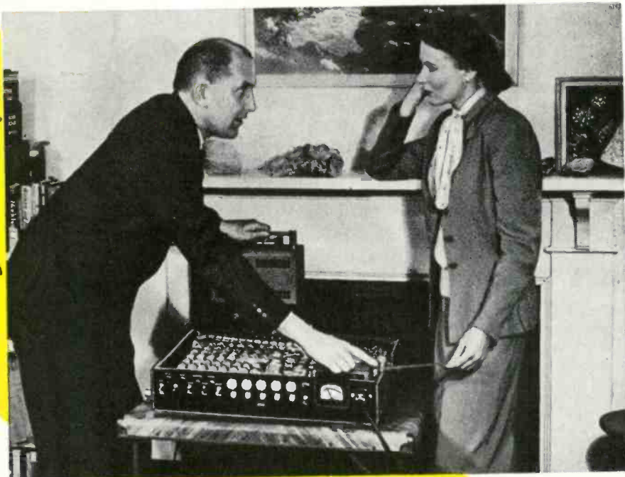
E. C. Berkeley explains how Simon gets instructions from a piece of punched tape.
