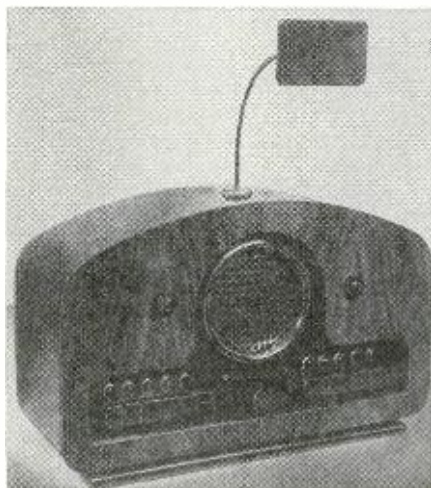
Body capacitance switches the intercom.
