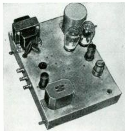
Parts must be mounted so as not to interfere with the turntable motor above.
