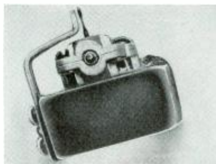
Fig. 4—This head-on view shows separation of the needle and copper strip.
