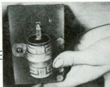
Filament battery is held by cable clamp.
