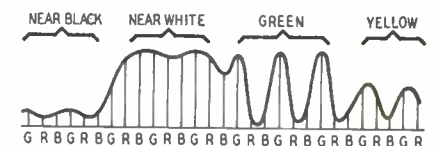
Fig. 4—Signal after passing through 4-mc filter. This is applied to modulator.
