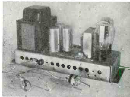
This is the power supply which furnishes low plate voltages for the tubes.
