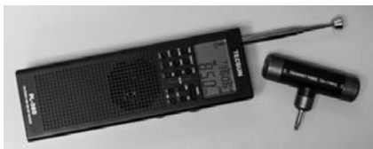
FIGURE 9 Another good AM/FM/SW portable receiver is the Tecsun PL-360, available for about $50 (at the time of writing). This model includes a very sensitive “loopstick” directional AM antenna.
