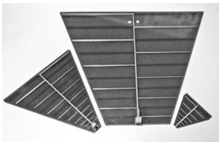
FIGURE 18 The larger PC board log-periodic antenna from Kent Electronics covers 400–1,000 MHz and costs under $30 (at the time of writing).
