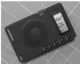
FIGURE 8 The Grundig “Mini-400” AM/FM/SW receiver is just $40 (at the time of writing) and makes a low-cost power line noise detector.
