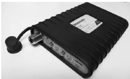
FIGURE 13 The Tektronix RSA306 USB-controlled real-time spectrum analyzer covers 9 kHz to 6.2 GHz and has a real-time bandwidth of 40 MHz. The cost is $3,489 (at the time of writing).
