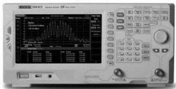
FIGURE 11 The Rigol DSA815 is an affordable spectrum analyzer that covers 9 kHz to 1.5 GHz. The cost is just $1,295 (at the time of writing). (Photo courtesy Rigol Electronics.)
