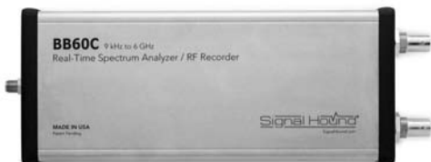
FIGURE 14 The Signal Hound BB60C USB-controlled real-time spectrum analyzer covers 9 kHz to 6 GHz and has a real-time bandwidth of 27 MHz. The cost is $2,879 (at the time of writing). (Photo courtesy Signal Hound.)
