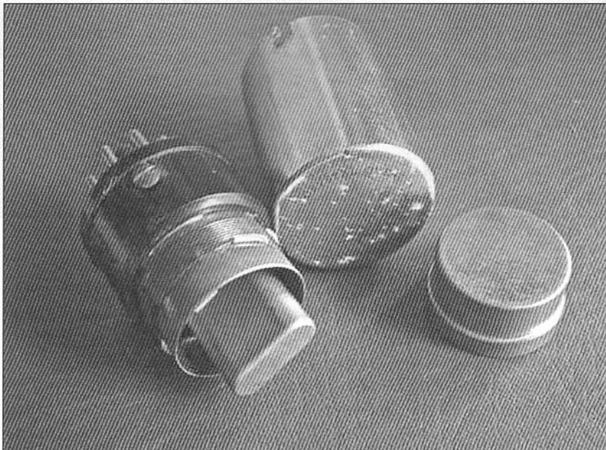
Fig 13.27: Cathodeon crystal oven for HC6/U crystals
