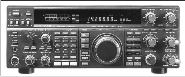
Fig 10.2: The Kenwood TS-850 is the most popular amateur bands transceiver used to receive on 136kHz
