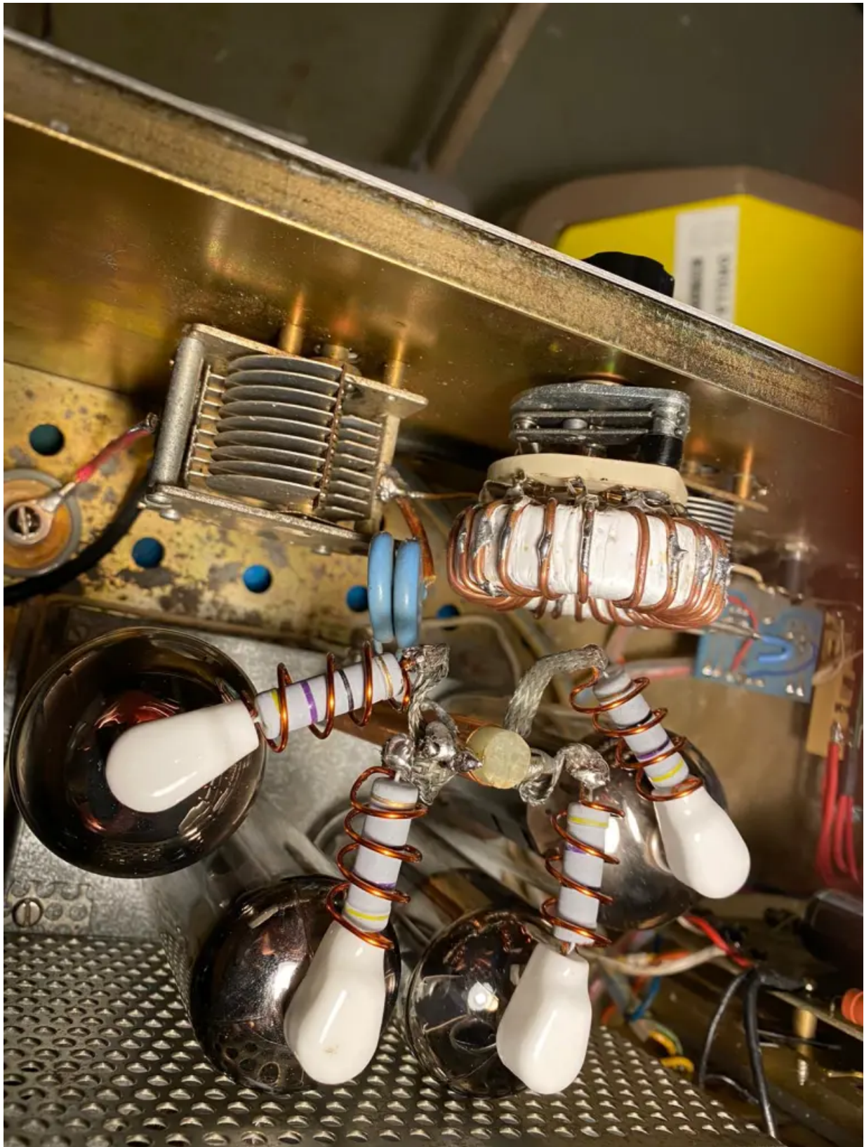
The PI NETWORK with a T200-2 Core
