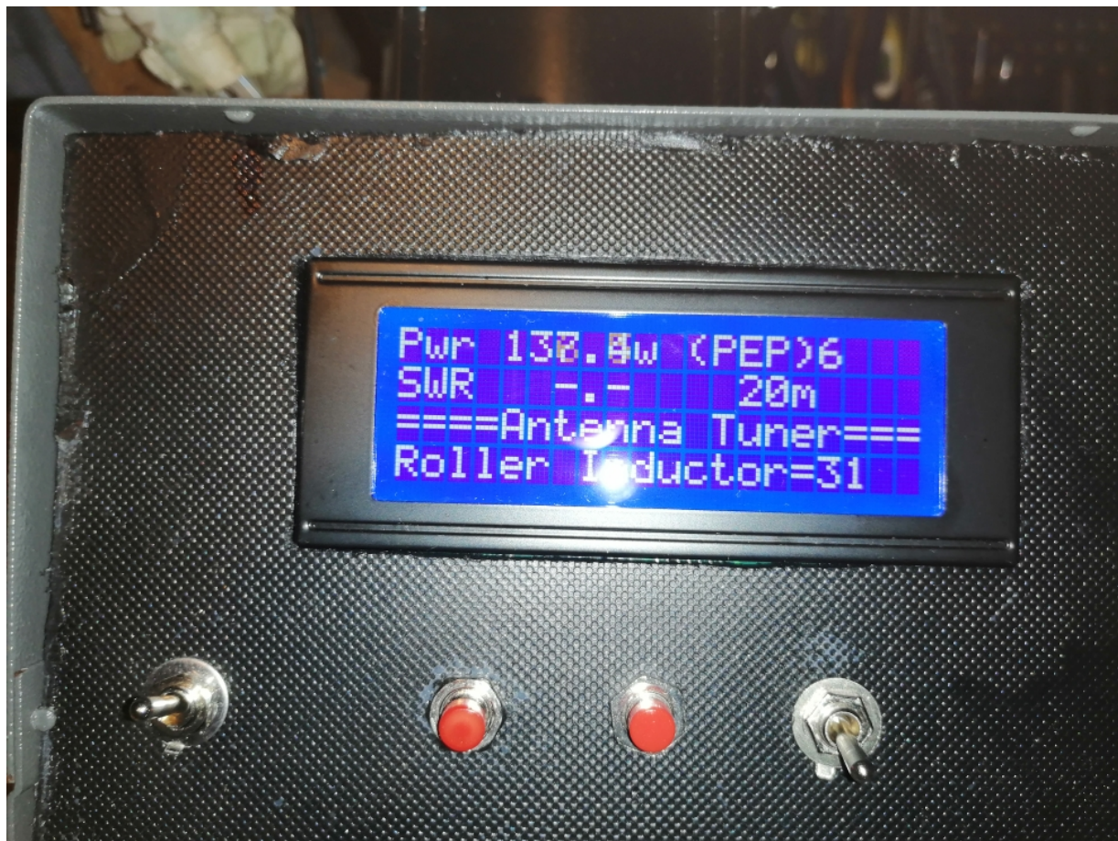
3w input 140w output on 20m
