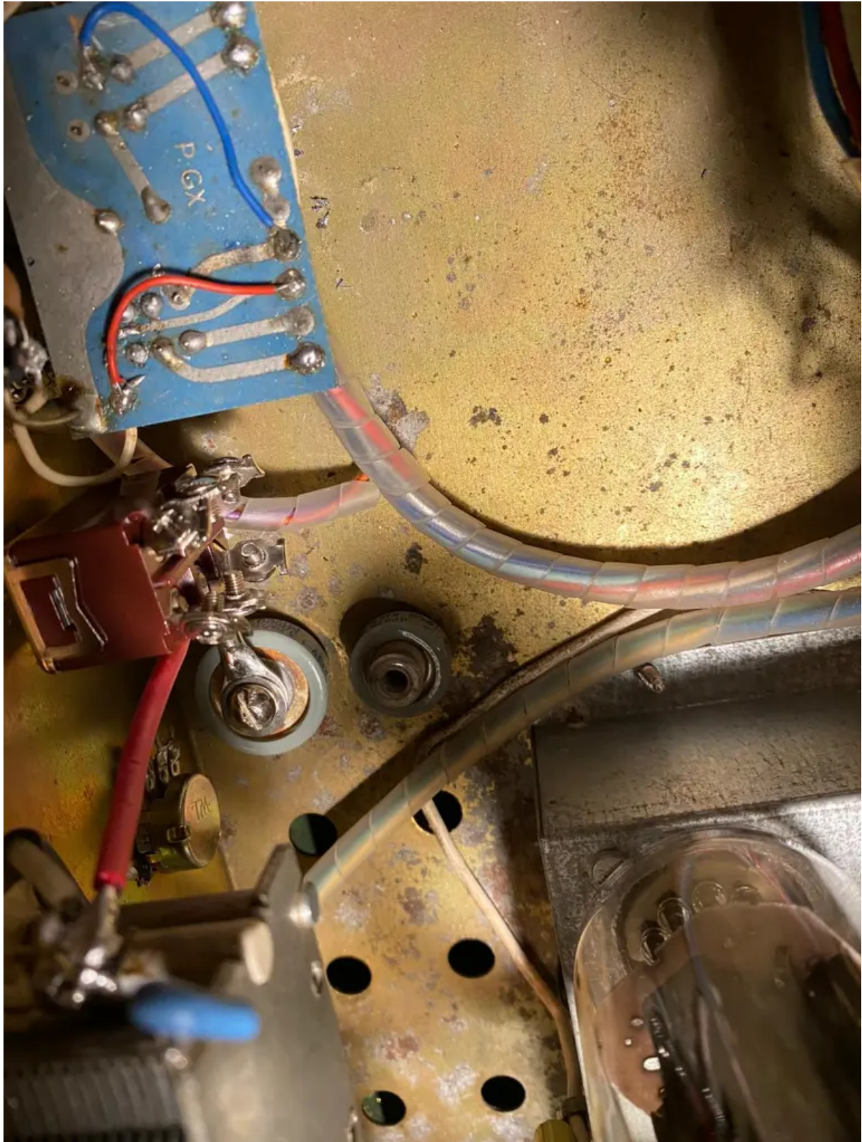
Additional 200 and 100pf capacitor at the Output of the PI Network
