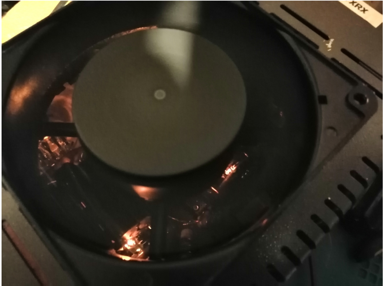
The Fan is on the top of the tubes (forced cooling with a 220vac fan)
