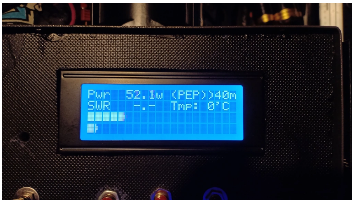
With about 1.5w input , this tiny amplifier is providing about 50w output. With 3w i can have about 70w
