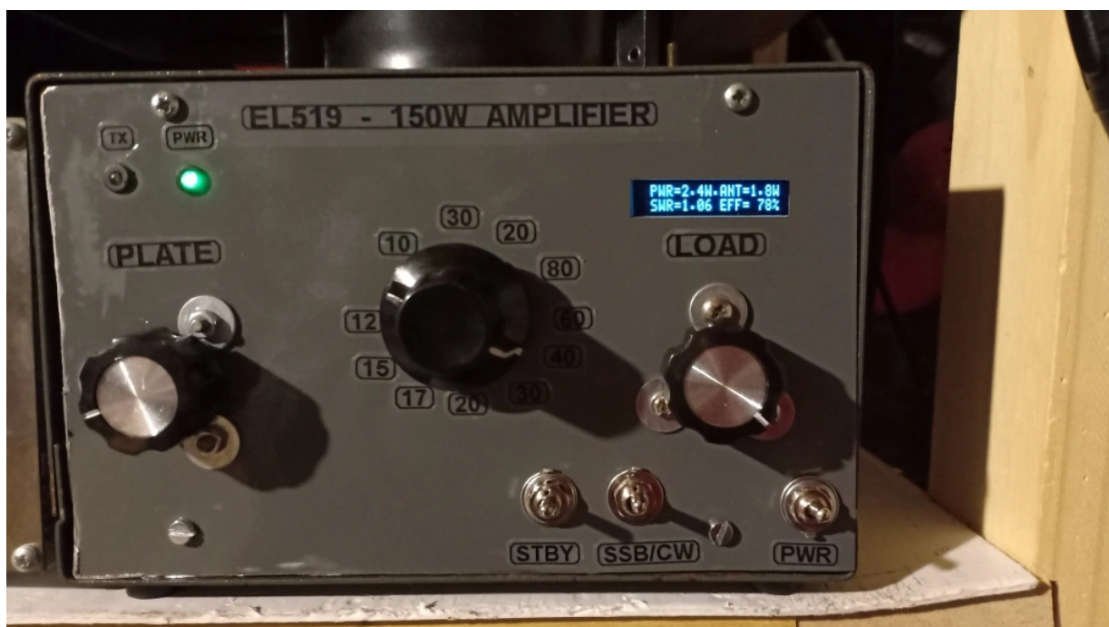
150W amplifier with one tube with N7DDC ATU display on the front panel
