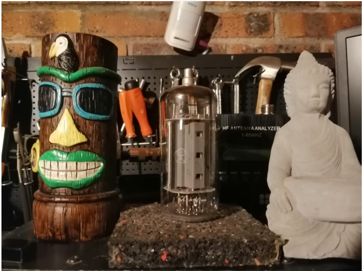
Tube 6P45S is a EL519 equivalent
