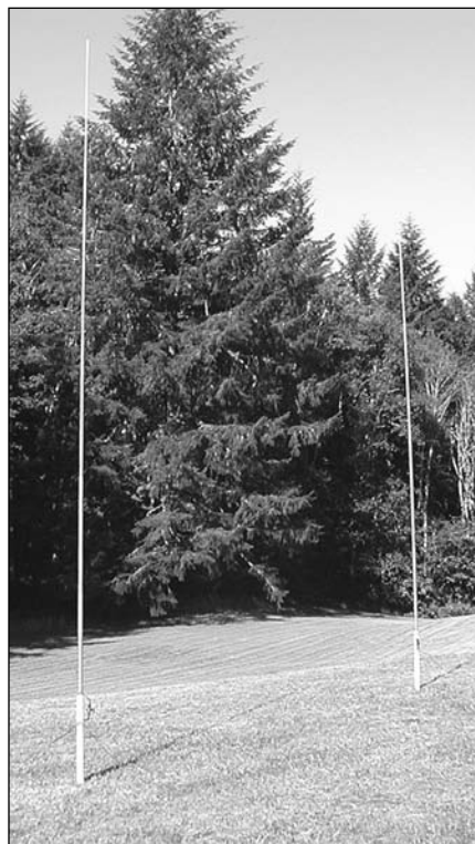
Figure 27.48 — 2-element 20 meter phased array (Photo courtesy N7MQ).
