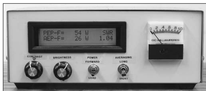
Figure 27.14 — Front panel of power meter. The LCD shows the peak envelope power (PEP), the average envelope power (AEP) and the SWR. The two knobs control the contrast and back lighting of the LCD. One toggle switch determines whether forward or load powers are displayed. A second switch sets the averaging time for the AEP calculation. The meter displays SWR and is used for tuning purposes.
