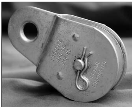
Figure 26.44 — A sturdy all-metal pulley suitable for tramming. (Photo by K4ZA)
