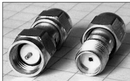
Figure 23.32 — A pair of SMA connectors, with male on the left and female on the right. SMA connectors are available in nickel, stainless steel, or gold finish.
