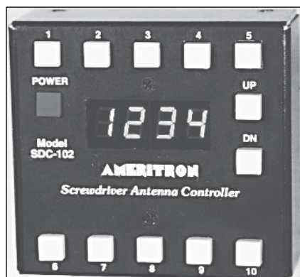
Fig 21.26 — A turns-counting controller keeps track of coil position by counting switch closures from a reed switch mounted on the antenna.
