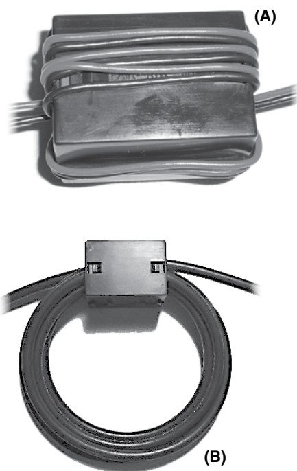
Fig 21.27 — At A, dc power leads are wound around a split ferrite bead to form an RF choke. B shows how coaxial cable can be wound on a split ferrite bead to form an RF choke on the outside of the cable shield. Wind coax loosely to avoid forcing the center conductor through the center insulation.
