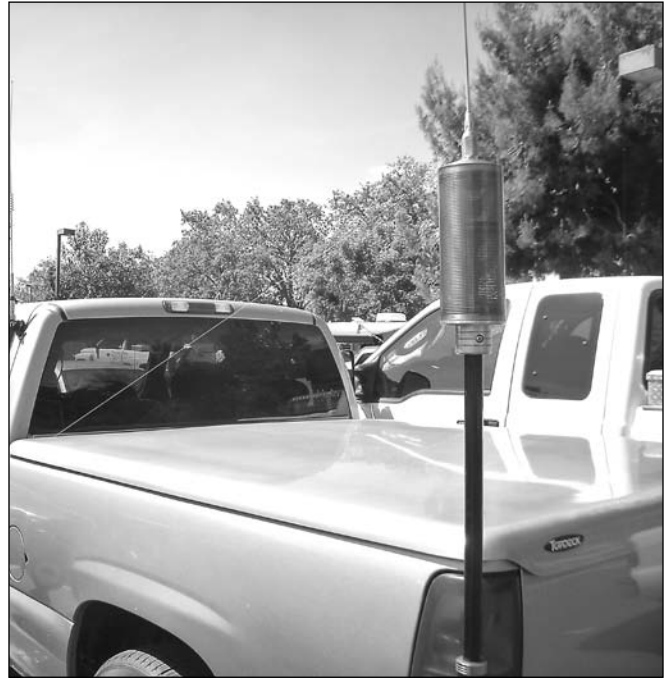
Fig 21.20 — A "bug catcher" style antenna showing the large, air-wound center-loading coil.
