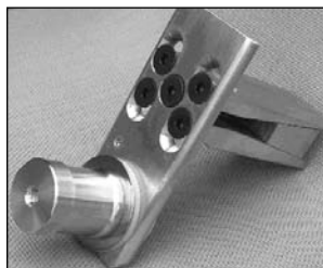
Fig 21.23 — Stake-pocket mounts are designed to fit into the square holes in the walls of a pickup truck's bed. An offset mount as shown in the photo will also clear most bed covers.
