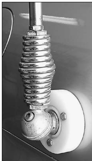
Fig 21.24 — A ball mount is attached to a vertical or nearly-vertical vehicle panel and can be adjusted so that the antenna is vertical. The spring shown in this photo may or may not be included with the mount. The length of the spring must be included in the antenna's total length.
