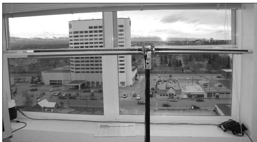
Figure 20.10 — This pair of CB mobile antennas were trimmed slightly to resonate on 10 meters then attached to a mounting bracket. This created an effective apartment-sized antenna.
