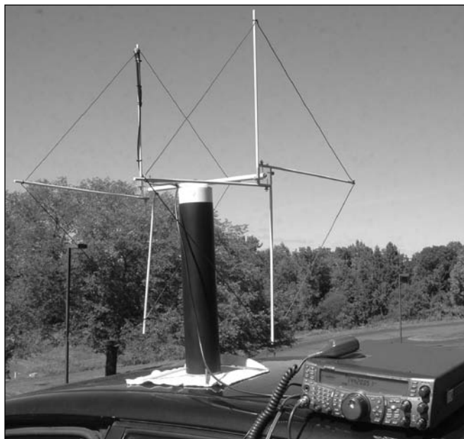
Figure 20.12 — The 2 meter PortaQuad by National RF isn't intended for permanent outdoor use, but it would be a fine directional antenna inside a room or attic.
