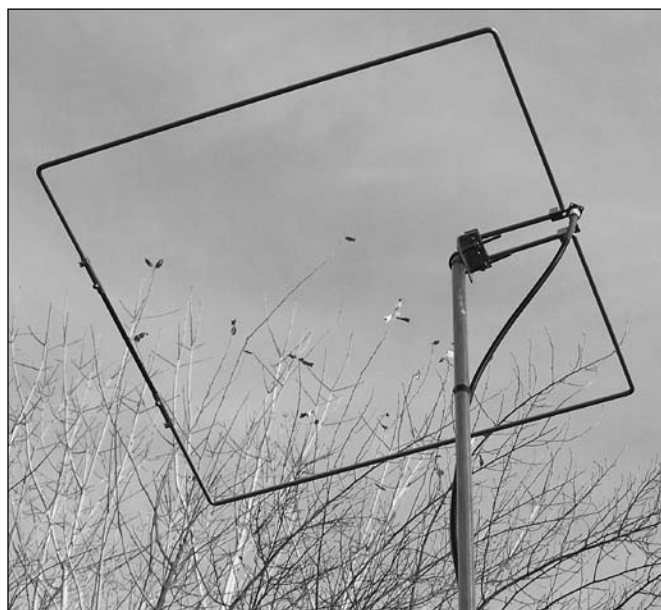
Figure 20.11 — A typical 6 meter horizontal full-wave loop antenna can be used either indoors or outdoors. The radiation pattern is omnidirectional with horizontal polarization.
