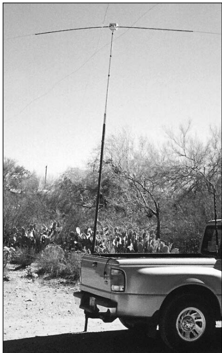
Figure 19.6 — A portable dipole made from a pair of mobile whip antennas. The mounting bracket can be home-made as in the article or purchased from a vendor of mobile antenna materials. Any suitable mast can be used.
