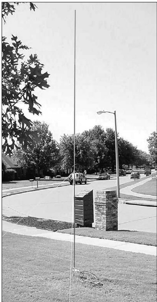
Figure 19.12 — The complete antenna set up in the author's front yard. Total height is about 16 feet.
