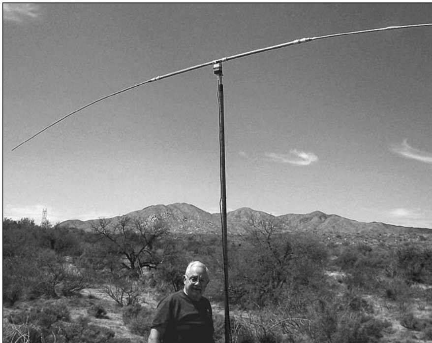
Figure 19.8 — This portable dipole uses a fixed center section and extendable telescoping whips to adjust the resonant frequency.
