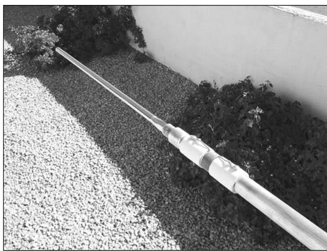
Figure 19.9 — One side of the antenna with the telescoped whip attached.
