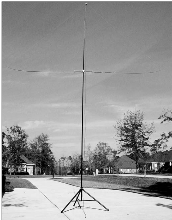
Figure 19.4 — The portable inverted-V antenna is built using a lightweight fiberglass support mast and two fishing poles. No additional supports are required and the antenna can be moved and rotated by hand.
