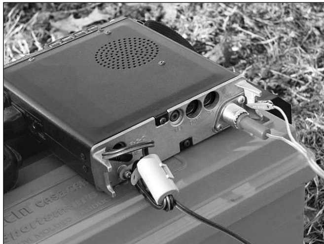
Figure 19.2 — Rear of radio showing banana plug and clip lead connections.
