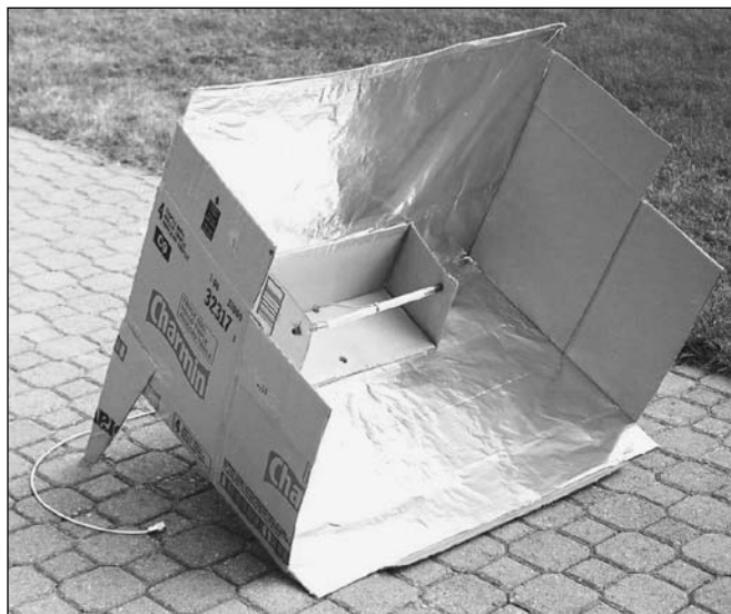
Figure 17.48 — The completed high-performance corner-reflector uplink antenna for U band. Note how the box corners hold the reflectors and dipole feed in place. The rear legs set the antenna elevation to 20° — this gives good coverage at the design latitude but will need modification for other stations.
