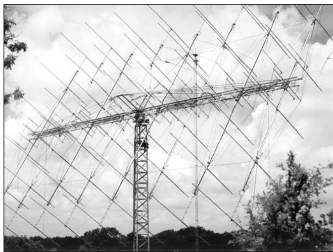
Figure 17.28 — K5GW’s huge 48-Yagi 2 meter EME array. (Photo courtesy K5GW)
