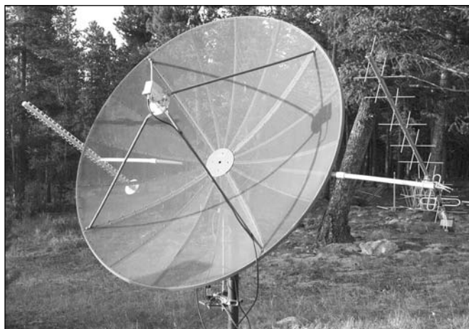
Figure 17.44 — WØLMD created this 8-foot dish with patch feed for S band for working HEO satellites. On the left is a helical antenna for L band and on the right is a 2 × 9-element offset-feed Yagi for U band. A homebrew az/el mount is provided. (WØLMD photo)
