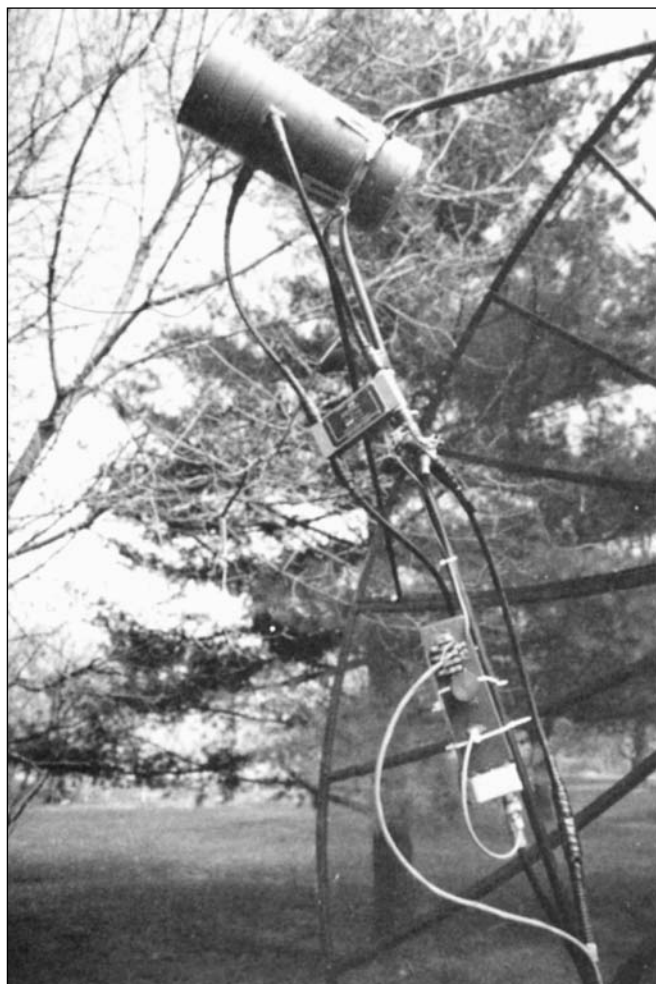
Figure 17.53 — View of feed, showing coffee-can feed horn and hybrid coupler.
