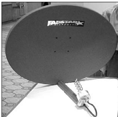
Figure 17.31 — PrimeStar offset-fed dish with KD1K's helix-feed antenna. N0NSV was so pleased with the modification that he re-named the dish "FABStar," and made a new label! (N0NSV photo)
