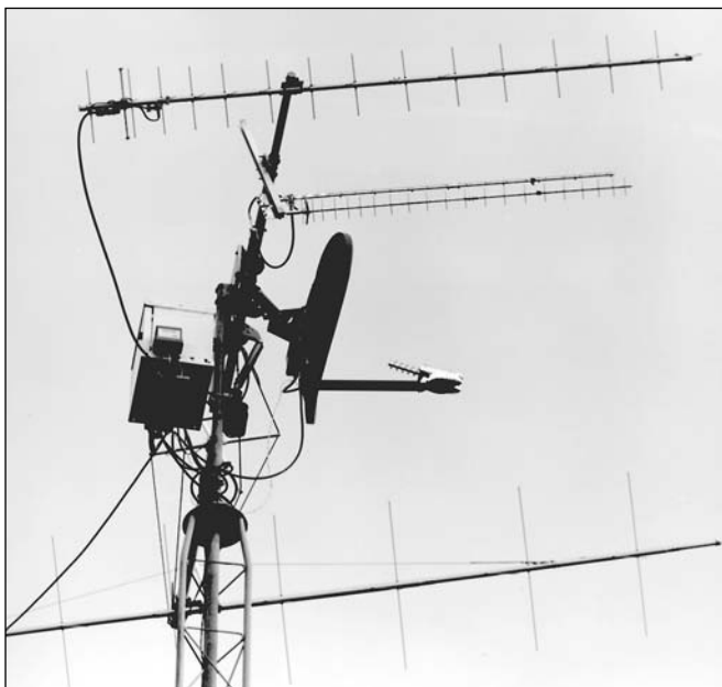
Figure 17.25 — Details of KD1K’s tower cluster of satellite antennas including a home-brew elevation rotator. Top to bottom: M2 436-CP30, a CP U-band antenna; two M2 23CM22EZA antennas in a CP array for L band; “FABStar” dish antenna with helix feed for S band; M2 2M-CP22, a CP V-band antenna (only partially shown.) To left of dish antenna is a NEMA 4 weatherproof equipment box with an internal 40-W L-band amplifier, and also hosts externally mounted preamplifiers. (KD1K photo)
