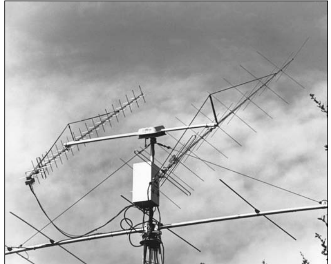
Figure 17.5 — Dick Jansson, KD1K, used these 2 meter and 70 cm crossed Yagis for HEO operations. The satellite antennas are shown mounted above a 6 meter long-boom Yagi.
