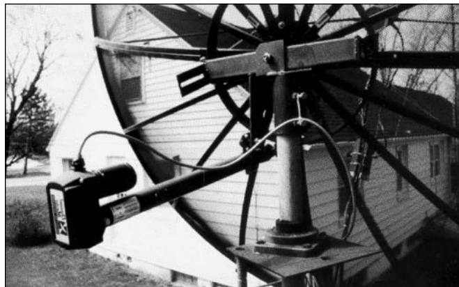
Figure 17.51 — Elevation system, showing modified TVRO mount.
