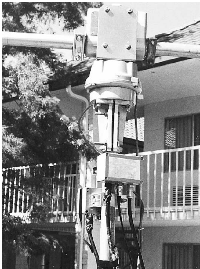
Figure 17.62 — At left, Yaesu az/el antenna-rotator mounting system is shown. Note that antenna loads must be more carefully balanced on this rotator than in the previously shown systems. At right, VE5FP has a solution for his az/el rotators by bolting two of them together as described in “An Inexpensive Az-El Rotator System” published in December 1998 QST .
