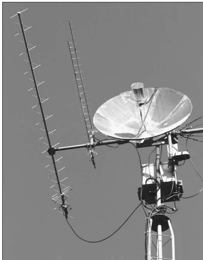
Figure 17.43 — KD1K’s completed HEO antenna system mounted to the tower and ready to go. The 40 W, 23 cm amplifier is in the box below the KG6IAL 1.2 meter dish. (KD1K photo)
