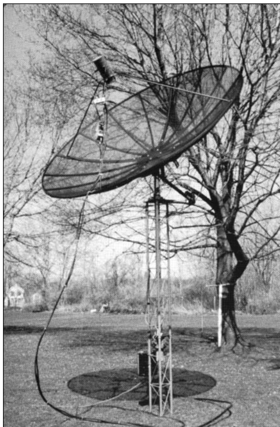
Figure 17.49 — View of K2DH's (ex-KD5RO) complete TVRO antenna installation. (K2DH photo)
