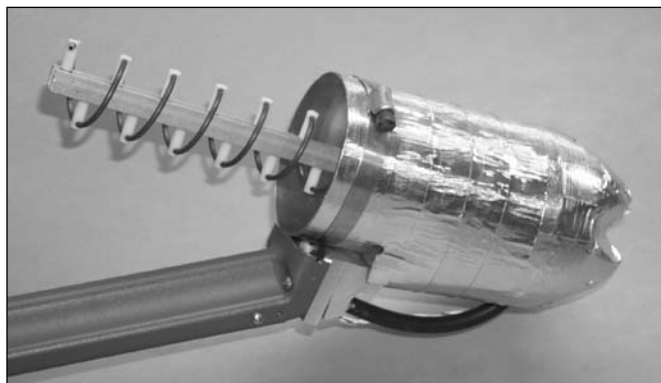
Figure 17.38 — Rain cover for preamp using a two-liter soft-drink bottle with aluminum foil tape for protection from Sun damage. (KD1K photo)
