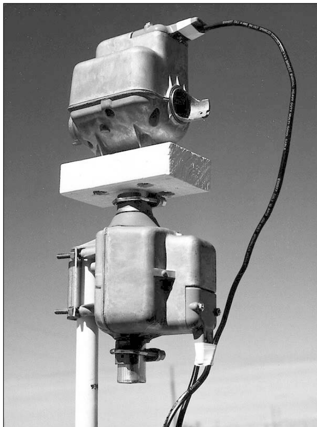
Figure 17.62 — At left, Yaesu az/el antenna-rotator mounting system is shown. Note that antenna loads must be more carefully balanced on this rotator than in the previously shown systems. At right, VE5FP has a solution for his az/el rotators by bolting two of them together as described in “An Inexpensive Az-El Rotator System” published in December 1998 QST .
