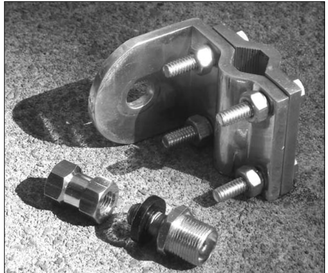
Figure 16.8 — The mirror-mount style of clamp-on bracket. This particular bracket is drilled for an SO-239 to 3/8-24 stud mount. The bracket can be mounted on vertical or horizontal struts.
