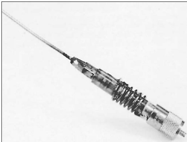
Figure 16.11 — The 222-MHz \frac{3}{8}\lambda mobile antenna. The coil turns are spaced over a distance of 1 inch and the bottom end of the coil is soldered to the coax connector.
