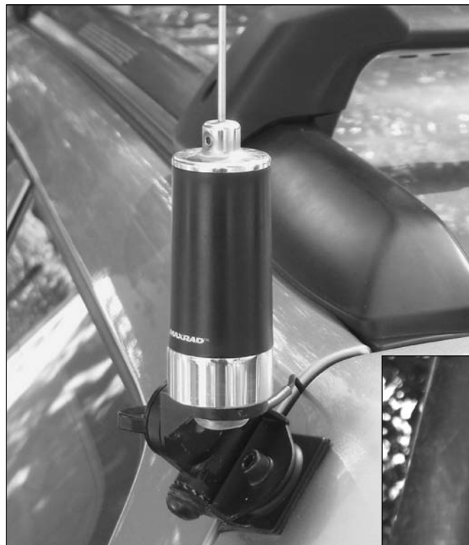
Figure 16.6 — (A) shows an adjustable lip mount made by Diamond. (B) is a close-up of the mount showing the set screws that hold the mount to the vehicle and make an electrical connection to the vehicle.
