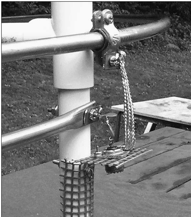
Figure 16.21 — Details of the feed connection. The main element could be mounted using the flattened tube approach instead of with clamps as shown.
