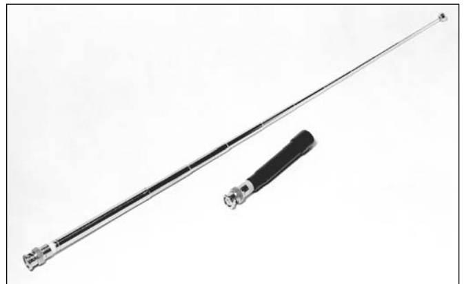
Figure 16.1 — A telescoping \frac{1}{4} -wavelength antenna and a “rubber ducky” antenna, both designed for use on 2 meters. The telescoping antenna is approximately 19 inches long when extended, while the rubber ducky antenna is only 3\frac{1}{2} inches long. The rubber ducky is a helically wound radiator used because of its mechanical strength.
