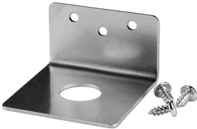
Figure 16.5 — This angle bracket mounts to the vehicle body with three sheet metal screws and is drilled to accept a standard NMO mount.
