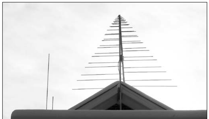
Figure 15.69 — The Tennadyne T-28 covers 50-1300 MHz with boom length of 12 feet.
