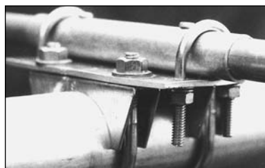
Figure 15.24 — The element to boom clamp. U bolts are used to hold the element to the plate, and 2-inch galvanized muffer clamps hold the plates to the boom.
