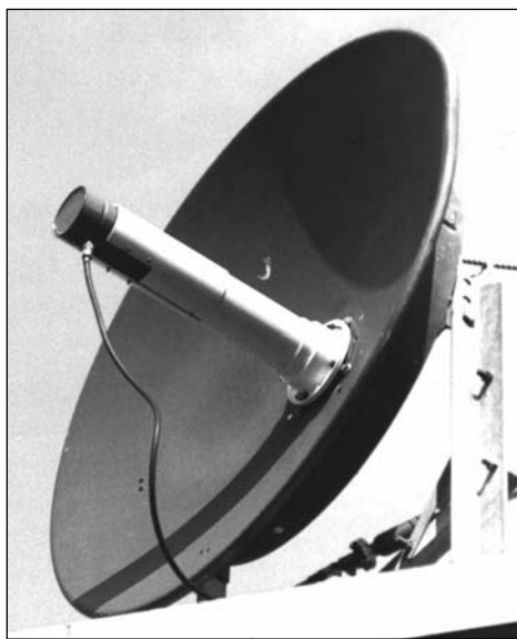
Figure 15.86 — Coffee-can 2304 MHz feed described in text and Figure 15.85 mounted on a 4-foot dish.
