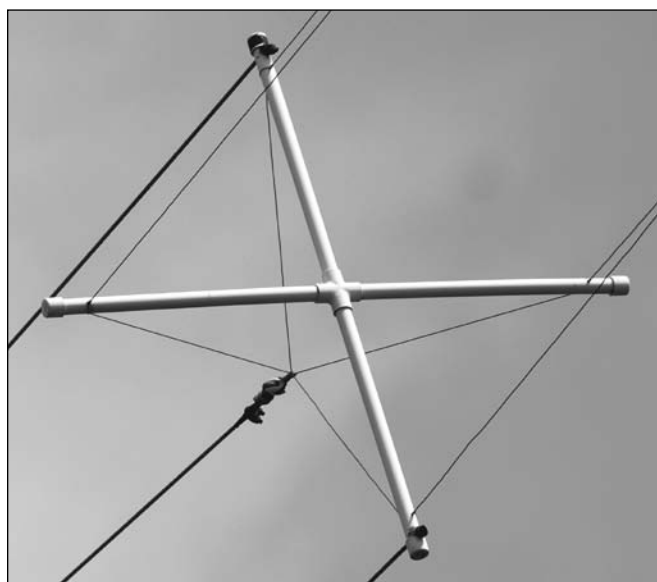
Figure 9.13 — The cage wires are kept separated by crosspieces of PVC pipe. The cage wires pass through a hole in the PVC pipe and a keeper wire is soldered to the cage wire on each side of the pipe to keep the crosspiece from moving along the wires.
