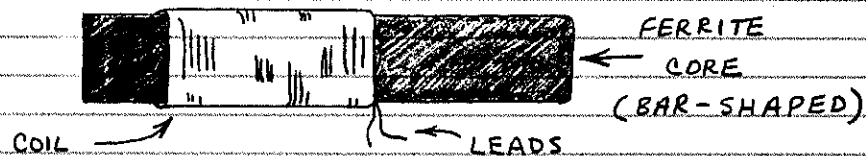
TYPICAL ANTENNA COIL
