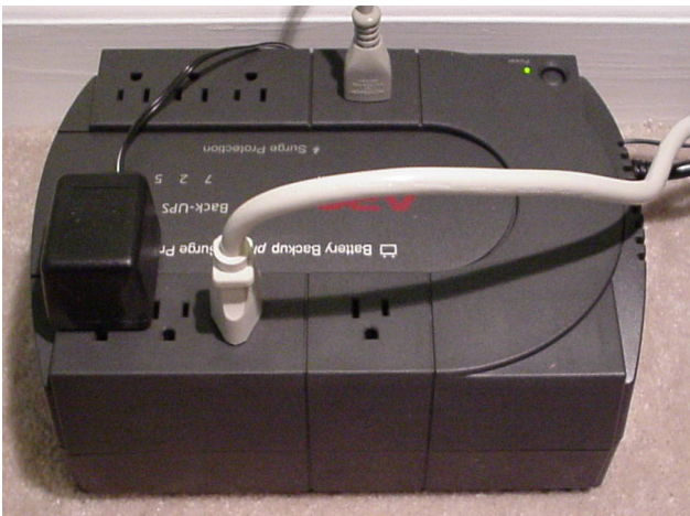
Figure 8.9 A UPS bought by the authors at an office supply store and used to provide backup power for a home computer. Although only 1/100,000 the size of the system in Figure 8.8, it is otherwise remarkably similar in design and purpose.
