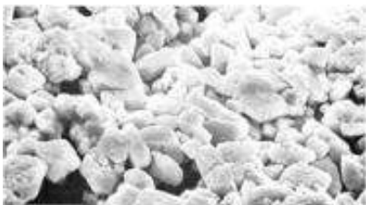
Figure 10-1: Crystalline formation on NiCd cell.
