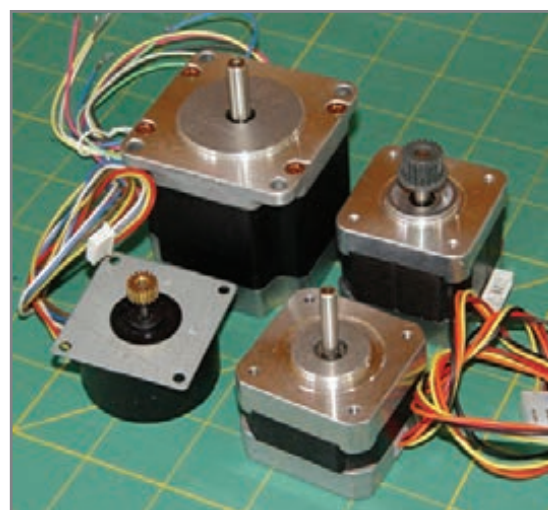
Photo 1 —This assortment of four-, five-, and six-wire stepper motors from my collection represents only a small fraction of the available designs. The largest motor is a NEMA 23 size, the two on the right are NEMA 17, and the smallest one, from my surplus heap, has a custom case.
