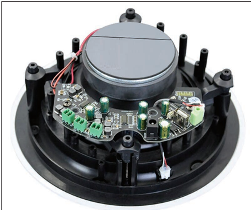
Photo 2: Here is a loudspeaker with an integral power amplifier.
