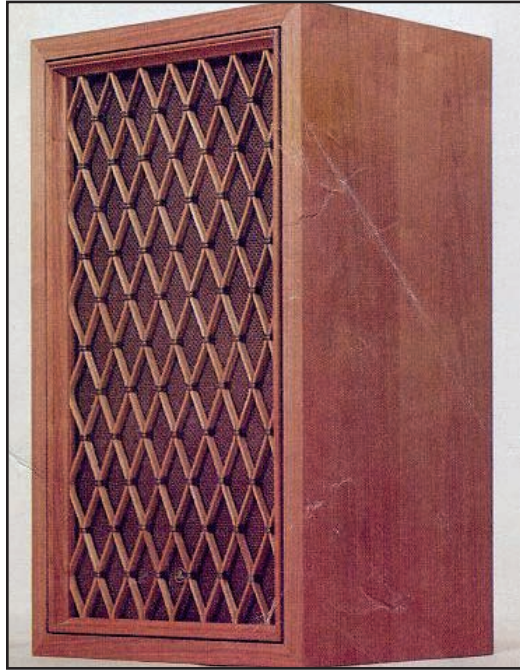
Pioneer CS-A77 Air Suspension speaker (late 1970s). Four-way speaker system with a 30cm woofer, a 12cm midrange, a 7.7cm tweeter, and a horn "super tweeter"—40Hz~14,000Hz, and 65W in a 75 liter box (17kg weight).
